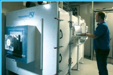
The flow characteristics of the Filterfans 4.0 were optimized during more than 1,000 tests in our modern test laboratory. The result: Modern, flat fins which enable maximal airflow, hold back dust and water particles, protect the filter medium from damage and can be integrated into the design of the applications.
